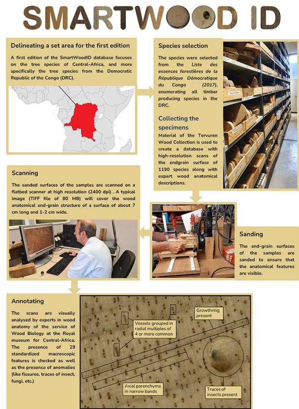
Figure 2. A flowchart showing the procedure of building the database.
