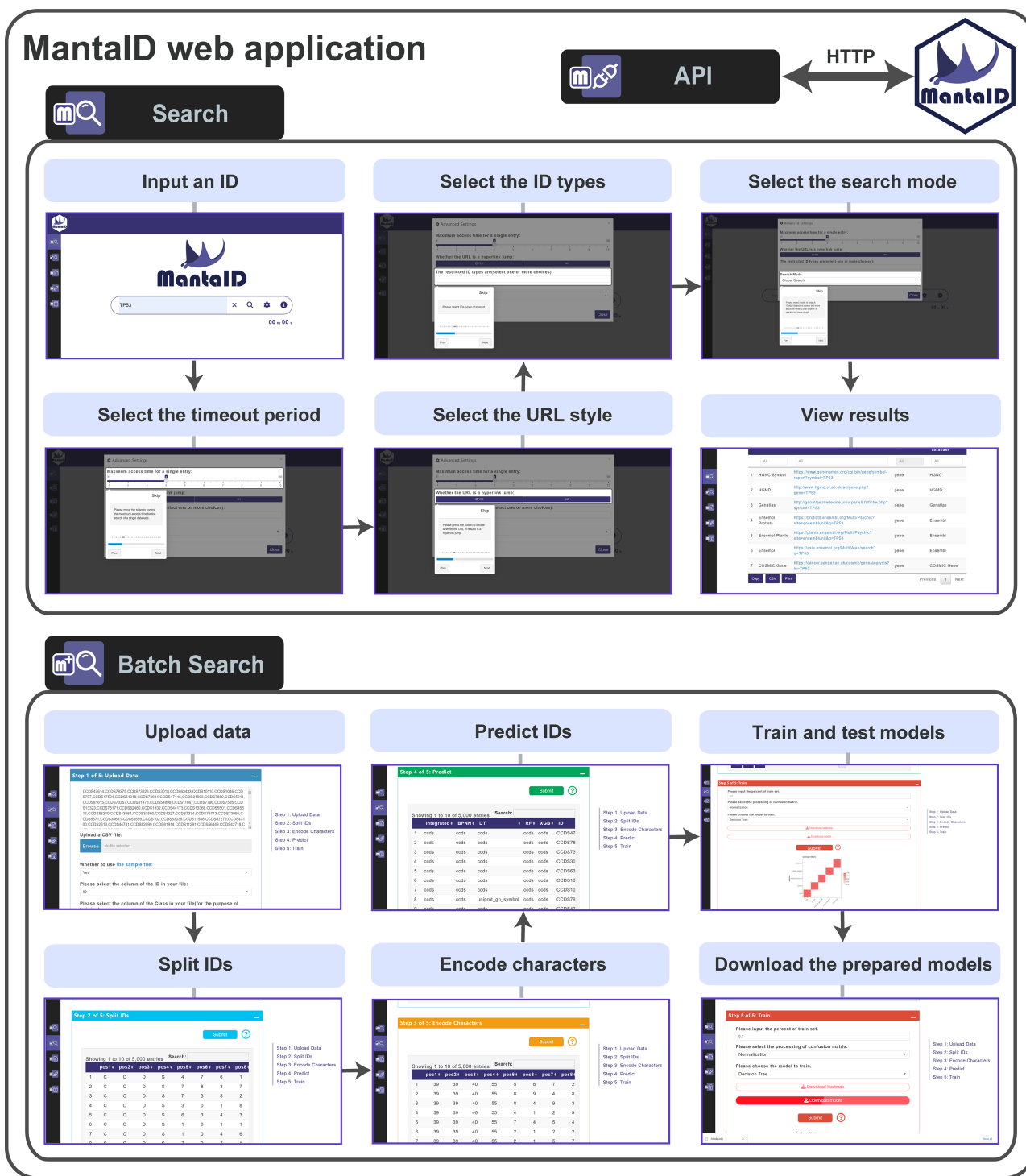
Figure 5. The features of the MantaID web application. The setting panels allow users to configure the basic and advanced settings; basic settings populate settings panels by default, whereas advanced settings enable a more granular control.
